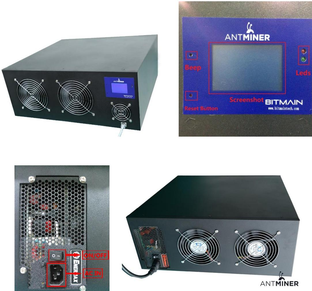
1000W PSU: when you set up AntMiner S2, only need to connect to AC 220V/50Hz or 110V/60Hz.
