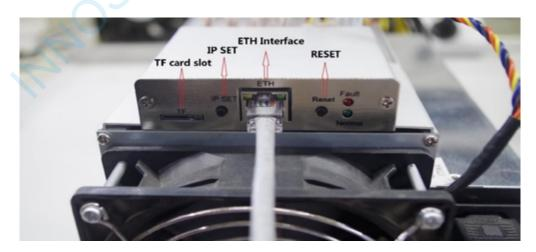
IP SET button: Press it more than 5 seconds to recover the IP to 192.168.1.254.
