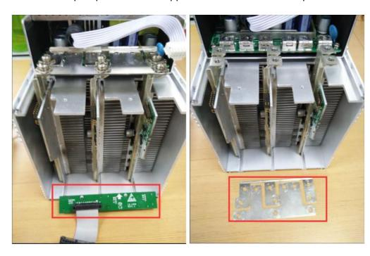
3) Extract the faulty hash board outward, as shown:
